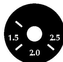
The positions marked on the potentiometer with 1.5, 2.0, 2.5 show the optimal current setting and the welding of the 1.5, 2.0, 2.5 mm electrodes.
